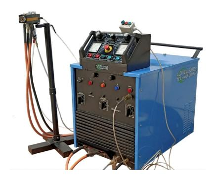
Offered twin wire arc spray system; Model: WST-8830/600-AR-JN combines typical features of the modern arc spray technology. The offered system operates on Pull Type principle wherein the wire is pulled by the electric arc gun roller which is driven by a pneumatic air motor.
